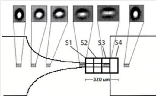
Illustration 4: The four sections used to measure RBC DIs, as well the deformation result of RBCs along the microchannel, adapted from [4].
