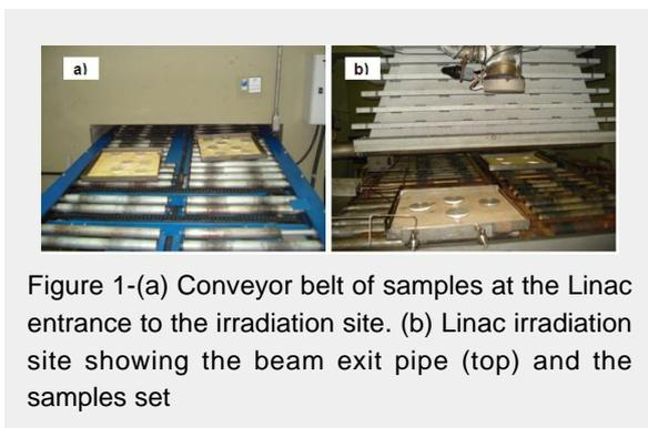
Figure 1-(a) Conveyor belt of samples at the Linac entrance to the irradiation site. (b) Linac irradiation site showing the beam exit pipe (top) and the samples set
